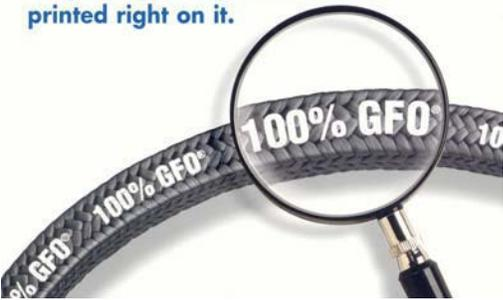
ROBCO 1140 compression packing is produced from a high tensile modulus PTFE (polytetrafluoroethylene) yarn into which a high percentage of micronized graphite and a small percentage of dimethylsiloxane (silicone lubricant) is added. GFO<sup>®</sup> fibre's combination of micronized graphite and silicone lubricant in the PTFE yarn resulted in a packing that retains nearly all of pure PTFE's chemical resistance while operating at pump speeds up to 4,000 fpm in cool liquids.
