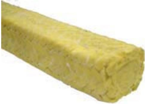
ROBCO 4029 is an all polymer aromatic polyamide fibre. The yarn possesses excellent static and dynamic fatigue resistance as well as a negative coefficient of expansion unlike other polymers such as PTFE (polytetrafluoroethylene) which expands at several times the rate of metals. The yarn is pre-lubricated with a combination of colloidal PTFE and a silicone lubricant (dimethyl siloxane).
