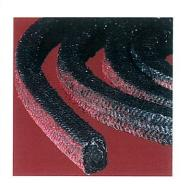
Enviropak 3450 is produced from a highest quality carbon core over which a double Inconel® wire inserted carbon yarn jacket is braided. The result is a stiff construction able to withstand high pressure. It will provide excellent performance in super heated steam. Enviropak 3450 is the perfect packing for air or motor activated valves when constant cycling demands the best.
