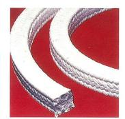
Enviropak 1121 is a thermally stable, chemically resistant, dry white PTFE fiber packing that will not harden or shrink in size in any valve service meeting Valve Manufacturer's Association specifications.
