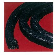
The carbon fiber in Enviropak 1000 is saturated with a PTFE suspensoid before and after braiding. It is a cost-effective substitute for pure PTFE, graphite and the higher grade carbon fiber packings. Enviropak 1000 is ideal for use in bleaching agents and cooking liquors in the pulp and paper industry.
