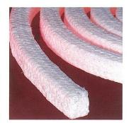
Each white, pure PTFE fiber is saturated with a colloidal Teflon® suspension before braiding. Then a high quality break-in lubricant is added to ensure thermal stability during start-up. Enviropak 1123 is an excellent choice on most chemical processes.
