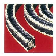
Enviropak 5079 is a GFO® fiber packing with Kevlar® corners. This combination gives you the heat dissipation of graphite filled PTFE with the high tensile strength of an aramid fiber that prevents roll and extrusion. Enviropak 5079 is the ideal choice on all equipment regardless of condition.
