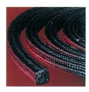
Enviropak 1140 is manufactured from 100% genuine GFO® yarn. It has excellent thermal conductivity and abrasion resistance. Enviropak 1140 is a great general purpose packing that will not hydrolyse and is unaffected by almost all chemicals.
