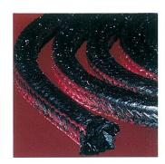
Enviropak 2000 is a thermally stable, high performance carbon yarn packing that is lubricated throughout with a combination of colloidal PTFE and graphite. Enviropak 2000 will not extrude, carbonize or soften as a Teflon® packing may. It is coated with a high quality breakin lubricant, offering outstanding resistance to steam and numerous chemicals such as aromatic alcohols, ketones, naphthenic hydrocarbons and solvents.
