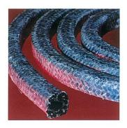
Braided from the best carbon yarn and completely lubricated with PTFE, Carpak is unaffected by strong caustic acids, or slurries. A standard packing for use in pulp and paper agitators, reactors, mixers and stock pumps.
