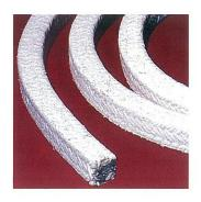
Enviropak 5050 is a cost-effective replacement for Teflon® impregnated Asbestos packing. The synthetic fiber is lubricated with a PTFE suspensoid before braiding. Our high quality break-in lubricant makes 5050 an effective packing for high-speed, rotary or reciprocating applications.
