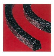
Thermograf is a resilient, compressible, self-lubricating, chemically inert, thermally conductive, braided flexible graphite packing . Once compressed, Thermograf 1200 becomes a totally homogenous ring that remains responsive to gland and system pressure changes. Thermograf offers optimum sealability from a braided packing for valves or pumps.
