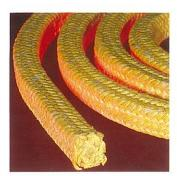
Enviropak 4029 is a high tensile strength extruded aramid fiber yarn packing for all abrasive applications. It is not recommended in steam or boiling water.
