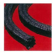
Enviropak 1342 is constructed of 99% graphite yarn impregnated with a micronized graphite lubricant. Superior performance can be expected in severe chemical conditions. It is an excellent choice for boiler feed, condensate or other high-speed rotary applications. The best heat dissipating qualities of any packing currently available.
