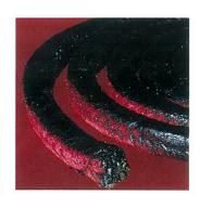
Enviropak 5019 is a low cost packing that performs well in a wide range of applications. It is made from synthetic yarn impregnated with graphite flake and, once braided, it is coated with a high temperature, break-in lubricant. Enviropak 5019 is effective on medium-speed rotary shafts.
